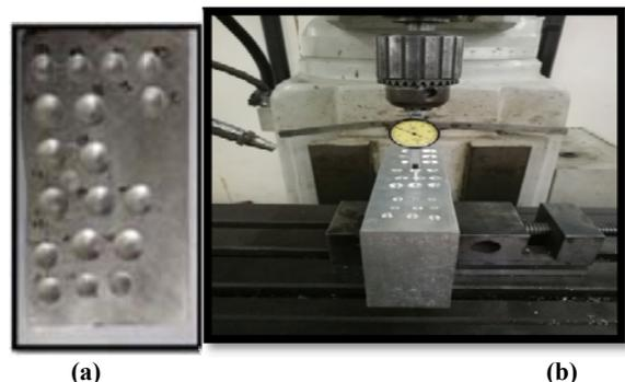
**Figure 2: (a) Drilled Workpiece; (b) Burr Height Measurement.**
