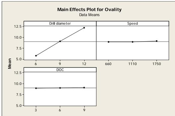
Figure 4: Input parameters vs Overcut (Ovality)
